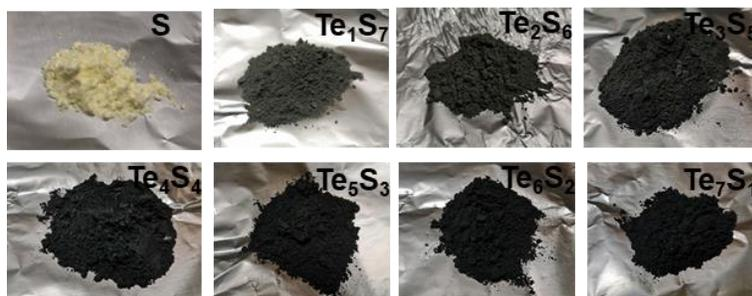
**Figure 6.1.1.** Digital photos of Te&S mixtures after ball milling.
